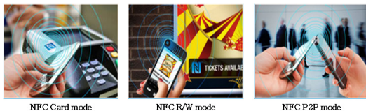
[Fig. 1] Three operation modes of NFC
