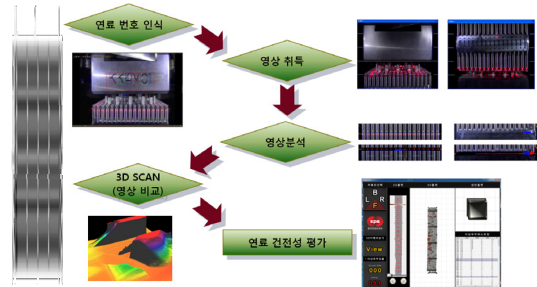
[Fig. 2] Inspection procedure of fuel assembly
