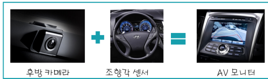
[Fig. 1] Reverse Parking Guidance System
