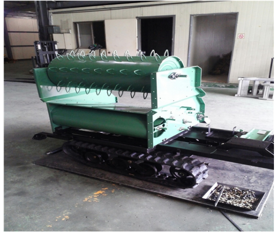
[Fig. 14] Assembling the threshing machine
