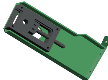
[Fig. 3] Support of the belt shaft
