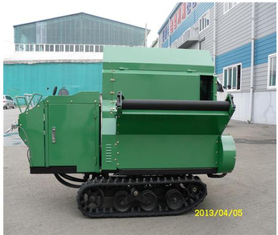
[Fig. 15] Prototype of the threshing machine
