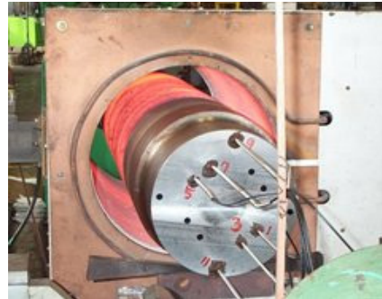
[Fig. 3] Induction Heating Equipment
