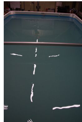
[Fig. 10] Lab water tank under turbidity of 26.4NTU
