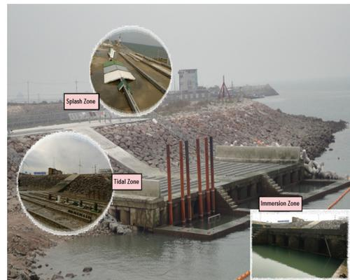
(b) Marine environment exposure test
