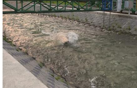
[Fig. 7] Failure process after limit velocity(underwater casting)
