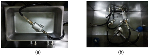
[Fig. 13] Test equipment (a) leak test (b) internal pressure test
