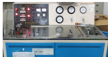
[Fig. 12] Impulse testing equipment
