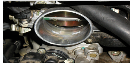
[Fig. 7] After cleaning throttle body
