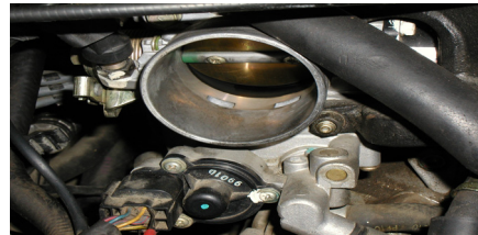
[Fig. 6] Throttle body before cleaning
