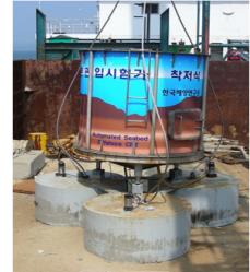
[Fig. 2] Seabed type offshore CPTU
