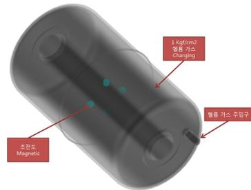
[Fig. 2] Structure of float
