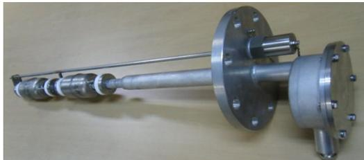
[Fig. 11] Prototype of level meter
