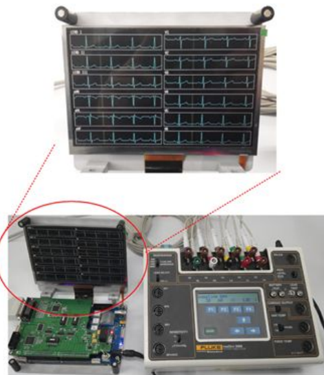
[Fig. 3] Result of 12 channel ECG Measurement system and test with patient simulator (mediSim300b, FLUKE)
