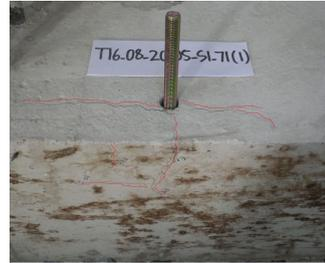
[Fig. 5] Failure mode (spitting and side-face blowout)
