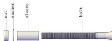
[Fig. 3] Figure of set anchor
