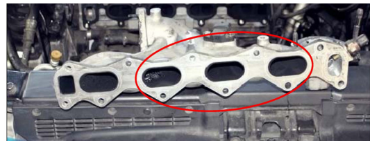
(a) Before cleaning the Intake manifold
