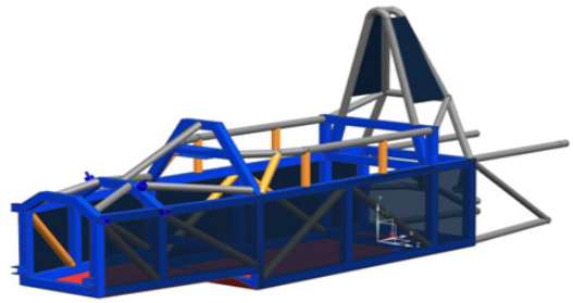
[Fig. 2] Initial 3D Modeling Feature of Frame Design
