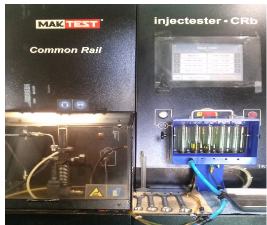
[Fig. 2] Injector test machine
