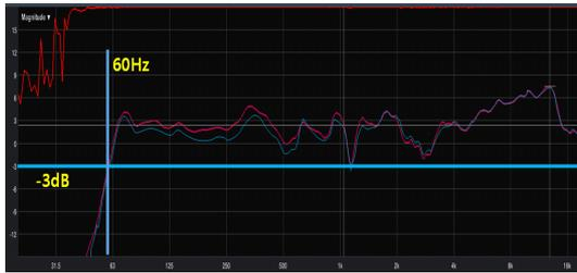
[Fig. 5] Comparisons of the frequency characteristics between the general type speaker and the magnetic type speaker with 2.4 ml
