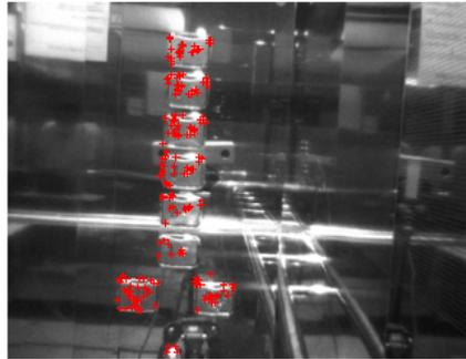
[Fig. 4] Elimination of reflected features
