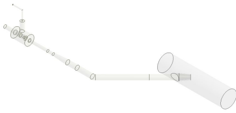
[Fig. 3] 3D modeling of flow region of Liquid-Gas Ejector.
