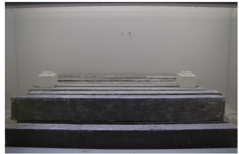
(b) Test specimens inside salt spray chamber
