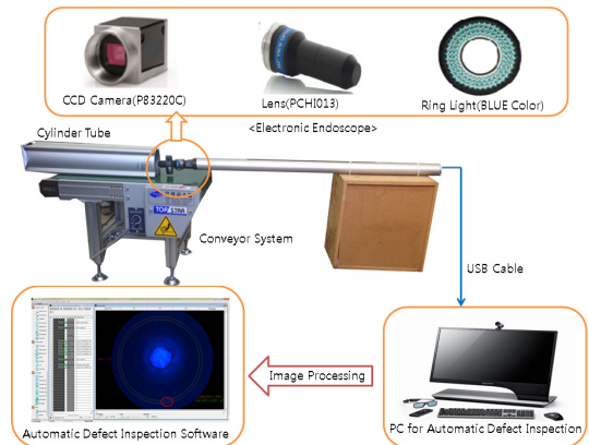
[Fig. 1] Configuration of automatic defects inspection system
