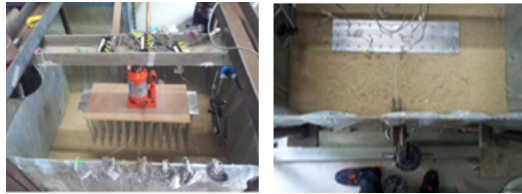
[Fig. 4] Installation of pile foundation
