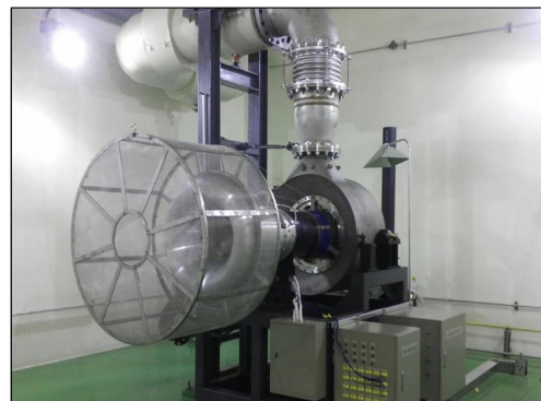
[Fig. 1] 200 kW Micro Gas Turbine under development
