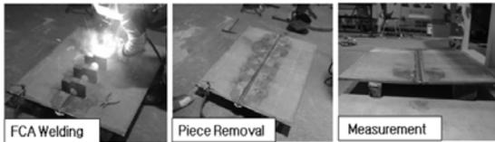
[Fig. 4] Procedure of experiments
