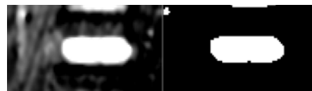
[Fig. 7] Example of binarization by Otsu
