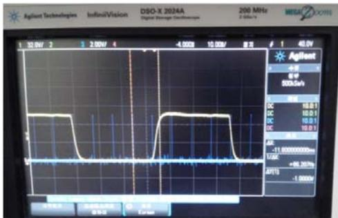
[Fig. 3] Response time measurement of WSS
