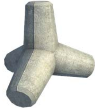
[Fig. 3] Wave dissipating block models for analysis (Tetrapod)
