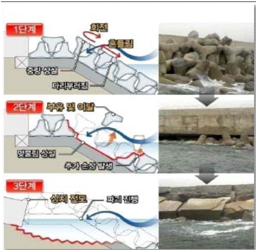
[Fig. 1] Behavior of wave dissipating block under wave load
