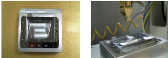
[Fig. 7] Gig and supersonic heating bonding machine
