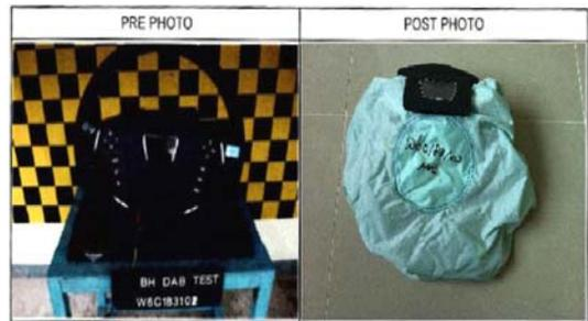
[Fig. 9] Digital LCD emblem system before and after airbag explosion test
