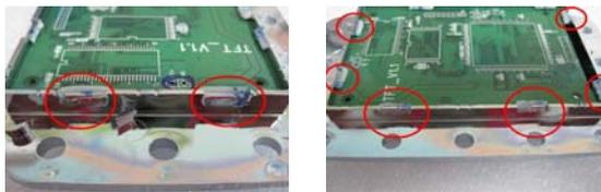
[Fig. 8] Supersonic heating bonding part of LCD assemble
