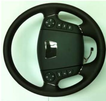
[Fig. 10] Steering wheel attached with digital LCD system
