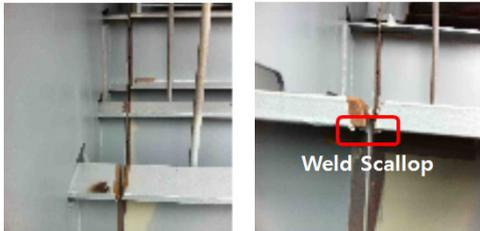
[Fig. 1] T-bar joint with weld scallop in block assembly stage
