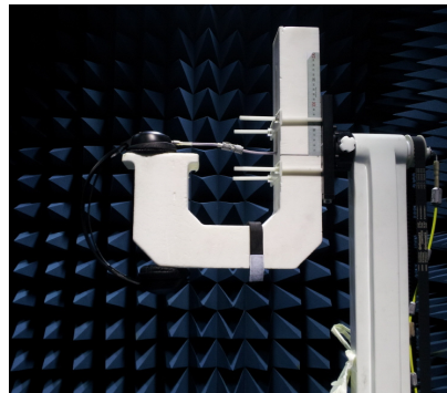
[Fig. 5] Photograph of measuring the antenna in the headset.
