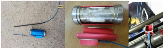
Fig. 1. Broken FBG(Fiber Bragg Grating) loadcell
