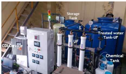
[Figure 1] Schematic diagram and Pilot plant of the LPM-CDI system
