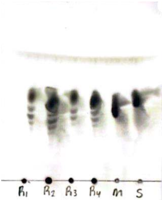
[그림 1] Results of an experiment to confirm the enzyme activity of dextransucrase via TLC. (* M: maltose, S: sucrose, * E1 strain culture temperature: 23 °C; E2 strain culture temperature: 36 °C )
