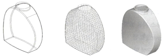
(a) Wire Frame model (b) Surface model (c) Solid model
