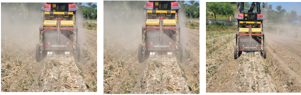
(a)PTO 750 (엔진 RPM 1600) (b)PTO 750 (엔진 RPM 1800) (c)PTO 750 (엔진 RPM 2000)
