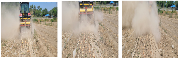
(a)PTO 1000 (엔진 RPM 1600) (b)PTO 1000 (엔진 RPM 1800) (c)PTO 1000 (엔진 RPM 2000)
