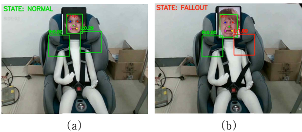
[그림 6] Results of AI-based detection models: a) Facial expression: Happy, Harness state: Normal; b) Facial expression: Sad, Harness state: Fallout (left arm ejected)
