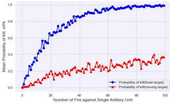
[그림 1] Comparison of Probability of killbetween Fixed and Moving Targets, fire range 10Km.
