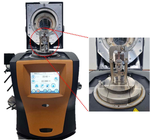
Fig. Photograph of the experimental setup for stress relaxation measurement of propellant of multiple rocket
