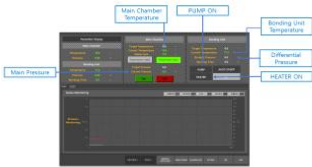
Fig. 2 LabVIEW-Based User Interface for the Automated Thermal Bonding System
